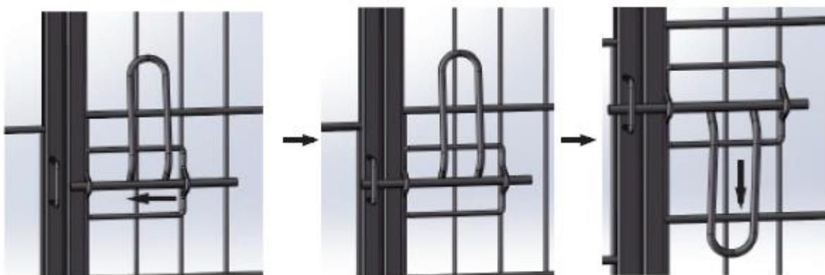
4) Close the door by sliding the handle bar through the hole in the lock.
