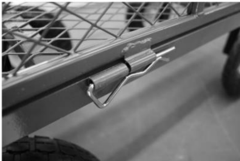
Figure 5: Mounting the side rails
