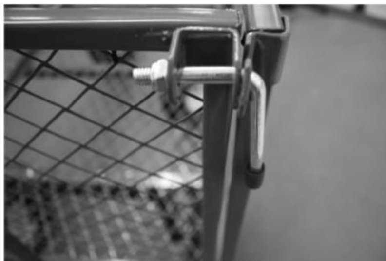
Figure 6: Mounting the "L-bolt"
