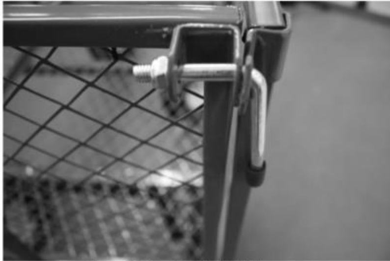
Figure 6: Mounting the "L-bolt"
