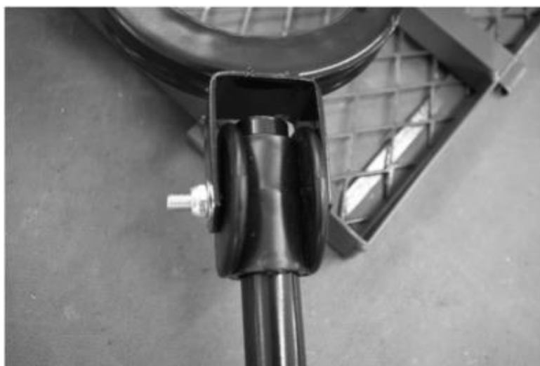
Figure 4: Mounting the handle
