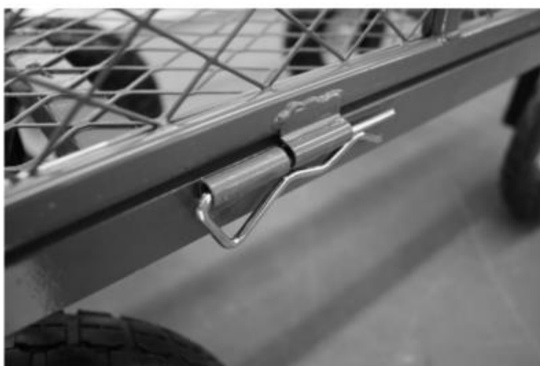
Figure 5: Mounting the side rails
